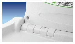
The unique hinge construction eliminates finger traps even during opening and closing. The hinge rotates within the enclosed moulding eliminating exposure to moving parts.
