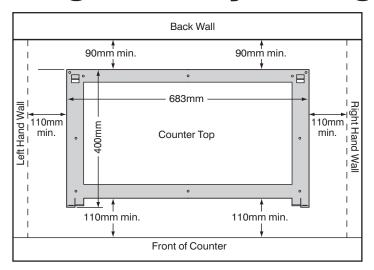
Position frame on counter top. Allow the minimum dimensions as shown.
